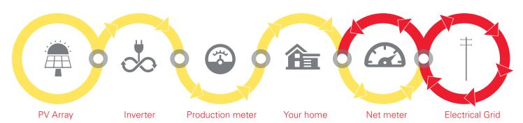
We read your net meter on a monthly basis to determine whether you're a net user or a net producer based on the kWh totals recorded on your net meter.
